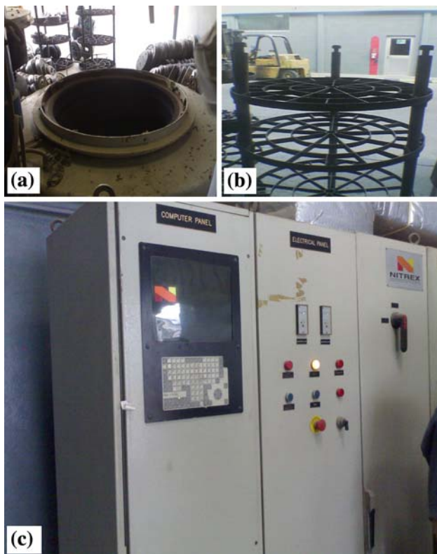
Fig. 3 Nitriding furnace, a top-loading design with a swing type cover (a) a “drain” of furnace for samples (b); process control hardware including process control, gas and electrical panels (c). Courtesy: Aluminum Products company, Dammam, Saudi Arabia
